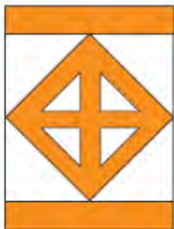
Type 5.11: Boating Restriction (NWPA) Size: a – 600mm x 770mm b – 900mm x 1150mm
