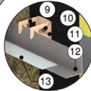
FERRO FAST Thermal Bracket System with Aerogel Coating
