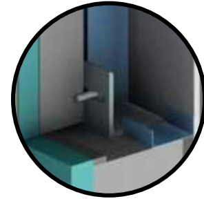
Gravity and Slot Anchor Detail
