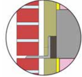
Insulation covers shelf angle for scenarios R-10+
