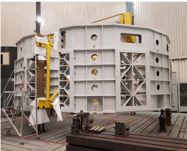
A stator frame sits ready to be shipped to BR2.
