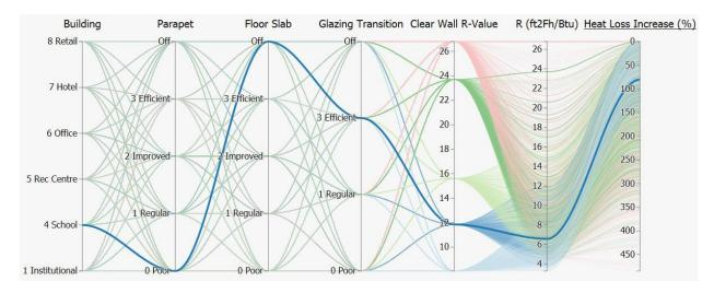
Figure 2 - Parametric Analysis of Base Building U-Value Impacted by Thermal Bridging
