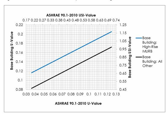
Figure 6 – Effective U-value Accounting for Linear Heat Losses for Varying Clear Wall U-vaues
