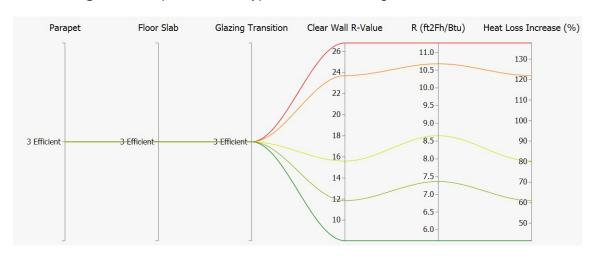
Figure 4 – Impact of Clear Wall on Heat Loss Increase over Base Building
