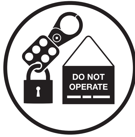
2. Ensure there is a Safety Protection Guarantee or Lockout in place and check that it is appropriate for your work.
