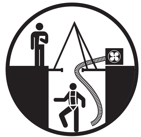
6. Maintain a safe atmosphere in a confined space and ensure you can be rescued.
