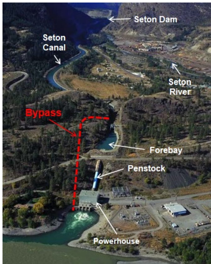
Figure 9 Alignment of the proposed Seton Bypass tunnel.
