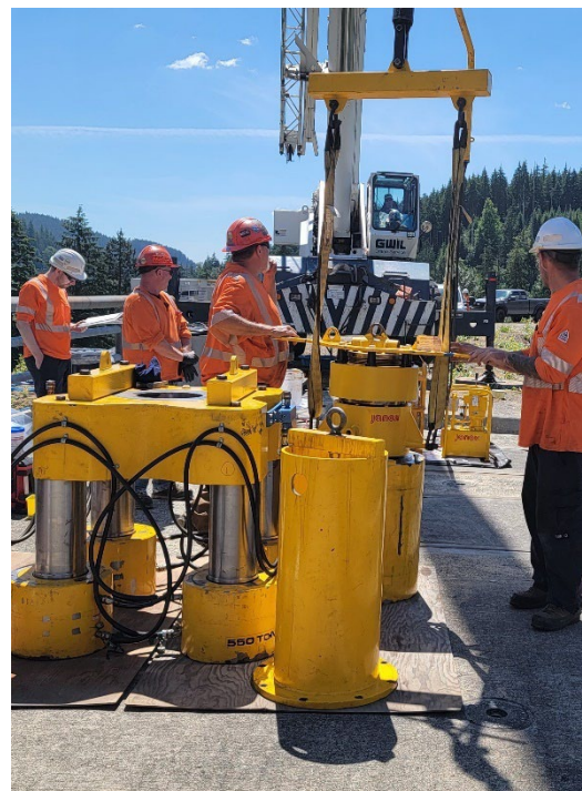
Figure 6 Above: Coquitlam Dam and the concrete transition structure. Right: Setting up the equipment to pull-test the concrete transition's three post-tensioned anchors.
