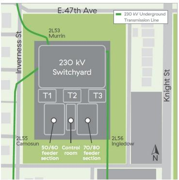
Figure 1 Mainwaring Substation Layout
