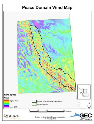
Wind speed adjustment of 20% was applied to a specific area to correct for persistent and significant underprediction of wind speed
