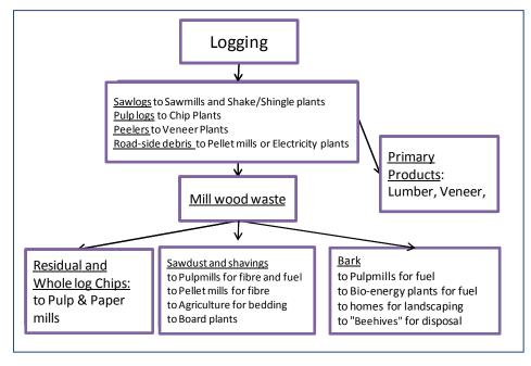
Figure 2. Basic Fibre flow Diagram
