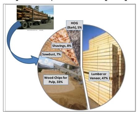
Figure 1. The Component Parts of an Average Sawlog
