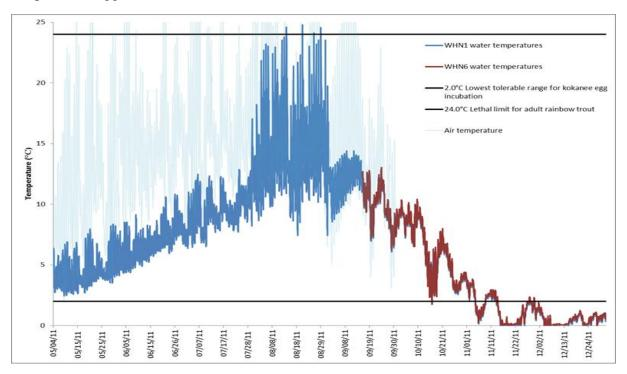
**Figure 6.** Water and air temperatures recorded from May to December 2011 at Site 1 from the WHN1 temperature logger, and September to December 2011 from the WHN6 temperature logger.
