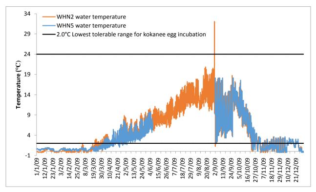
**Figure 10.** Water temperatures recorded from January to December 2009 at Site 2 from the WHN2 temperature logger, and January to June, and September to December 2009 from the WHN5 temperature logger.
