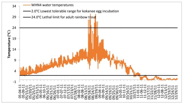
**Figure 19.** Water temperatures recorded from May to December 2011 at Site 3 from the WHN4 temperature logger. Data measured at 30 minute intervals.
