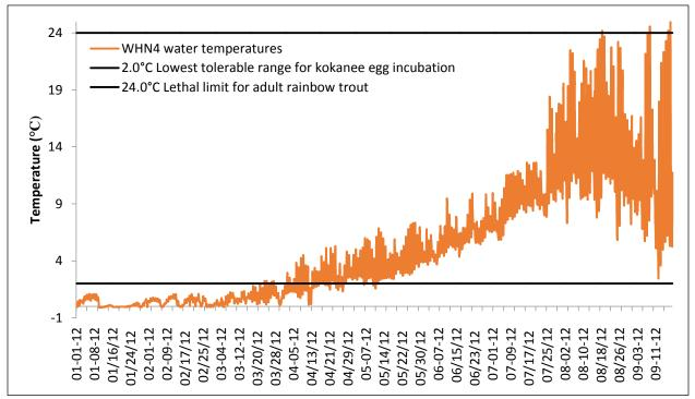
**Figure 21**. Water temperatures recorded from January to September 2012 at Site 3 from the WHN4 temperature logger. Data measured at 30 minute intervals.
