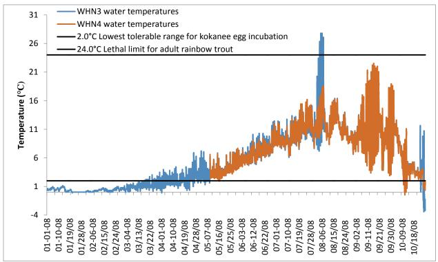
**Figure 15.** Water temperatures recorded from January to October 2008 at Site 3 from the WHN3 temperature logger, and May to October for the WHN4 temperature logger.
