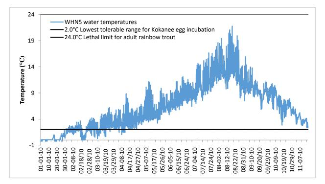
**Figure 11**. Water temperatures recorded from January to November 2010 at Site 2 from the WHN5 temperature logger.
