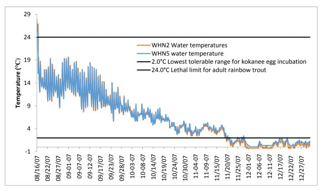
**Figure 8.** Water temperatures recorded from August to December 2007 at Site 2 from both WHN2 and WHN5 temperature loggers.
