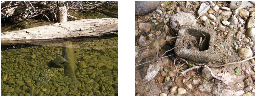
Figure 5.4.b: Temperature loggers in cinder block underwater and dewatered, Cranberry Creek, Sept 2009.
