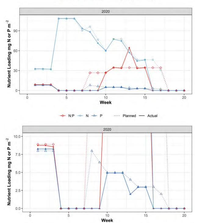
Figure 2. Upper figure shows seasonal planned and actual nutrient additions for Wahleach Reservoir, including areal nitrogen and phosphorus loading as well as molar N:P ratios, 2020; planned values are represented by hollow points and dashed line, while actual values are represented by solid points and solid line. Lower figure is zoomed in to better show phosphorus loading values.
