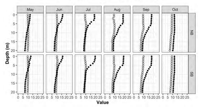
Figure 9. Water temperature (°C) and dissolved oxygen (mg·L-1) profiles at the north basin (NB-LS1) and south basin (SB-LS2) limnology sampling stations May to October, 2020, Wahleach Reservoir, BC.
