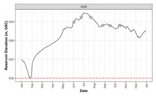
Figure 6. Daily reservoir surface elevation (m, Geodetic Survey of Canada), 2020, Wahleach Reservoir, BC. Open circles represent limnology sampling dates. The red dashed line represents minimum operating level of 628 m.
