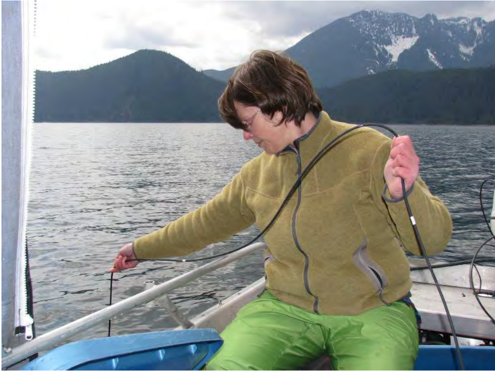
Figure 3.7 Light Intensity Profile Being Measured on Stave Reservoir
