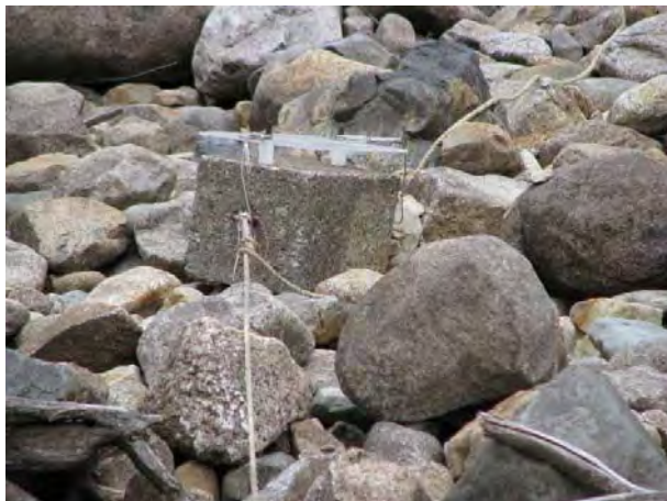
Figure 2.7 Concrete Littoral Sampling Block with Plate Attached (pre-2011)
