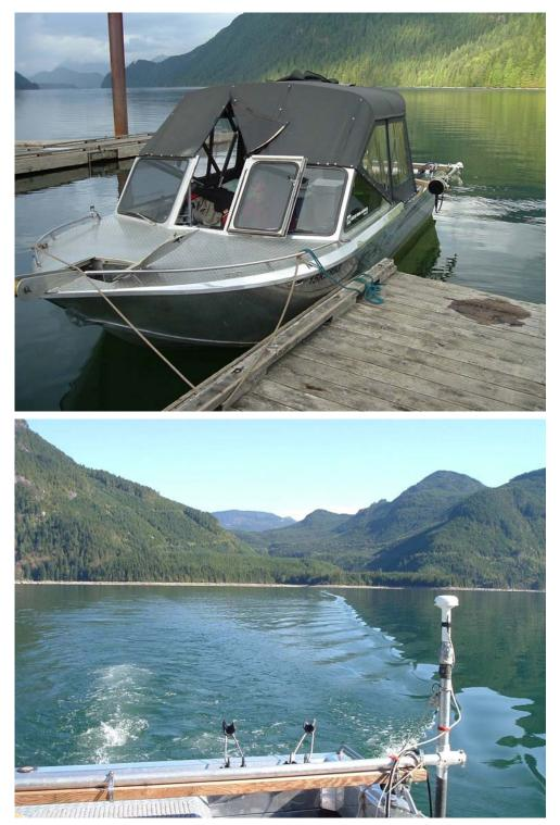
Figure 7. The acoustic sampling boat, with the pole mounted transducer out of the water for fast travel (upper) and in the water while sampling (lower).
