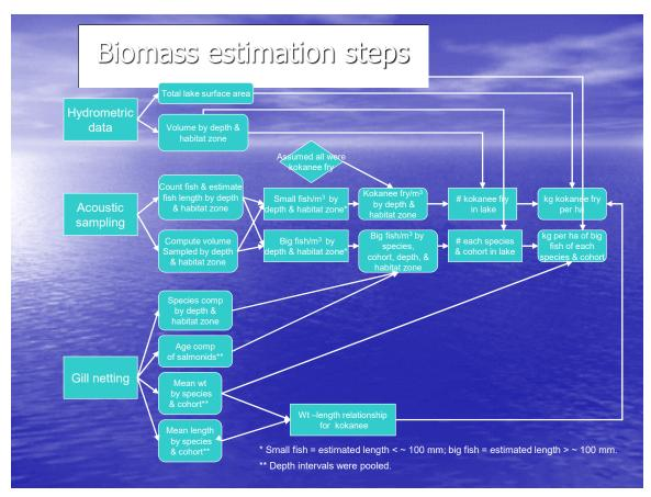
Figure 8. Schematic diagram of annual fish abundance and biomass estimation process.
