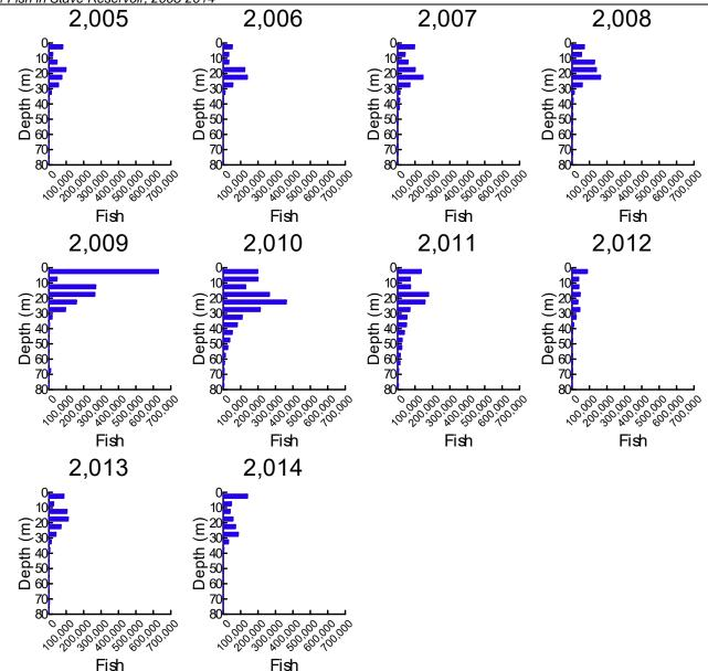
Figure 26. Acoustic estimate of total fish abundance (species and habitat zones combined) by 5 m thick depth intervals in each year of the 2005-2014 Stave Reservoir Fish Biomass Study.
