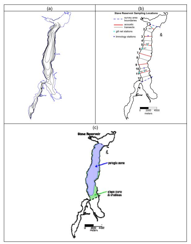
Figure 2. Maps of Stave Reservoir: a) bathymetric map showing the reservoir outline at full pool (82.1 m above sea level) with 10 m depth contours; b) the study area showing sampling stations and acoustic survey transects (main transects in bold red lines), and c) horizontal extent of the pelagic and slope/shallows zones within the study area.
