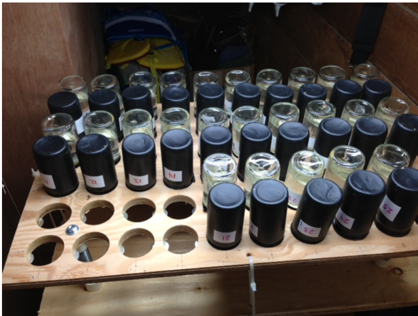
Figure 3.2: Shaker Table with light and dark bottles
