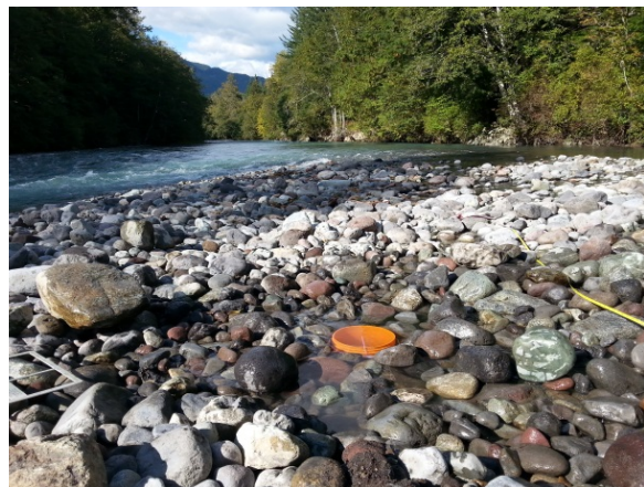
Photo 2: Trap is installed with lip of bucket flush with river bed.
