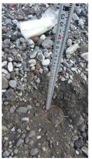
Photo 3: Sediment trap in bar top at Eagle Point also buried under ~30 cm of sediment following Jan. 2016 discharge event.
