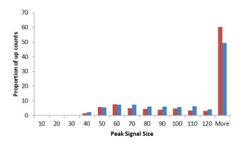
**Figure 14**: The proportional distribution of peak signal size for up counts recorded at BC Rail (blue bar) and Upper Paradise (red bar) spawning channels during the 2010 monitoring season.
