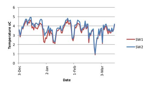
**Figure 18:** Cheakamus River water temperature in degrees Celsius recorded by two separate loggers (SRW #1,2) from December 3, 2010 to March 17, 2011. Water temperature was recorded 0.30 (m) above the river substrate in two stilling wells proximate to the spawning area near Moody's Beach (RKM 3.5).
