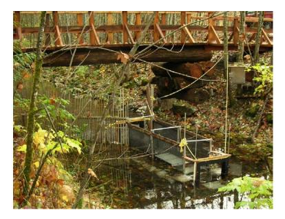
**Figure 5**: BC Rail side channel enumeration site. Upstream migrant spawners pass through a counter flume with a resistivity counter pad (white) and two 0.5 x0.5 m square full-duplex PIT detection antennae (black).
