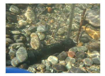
**Figure 8**:<u>TOP</u> – water temperature logger becomes incorporated into a capped 30cm section of perforated PVC pipe to form a simulated egg capsule. <u>BOTTOM</u> – one of nine capsules is anchored and then 6 reburied into randomly selected chum redds near Moody's Beach and 3 at the Gauge Pool.
