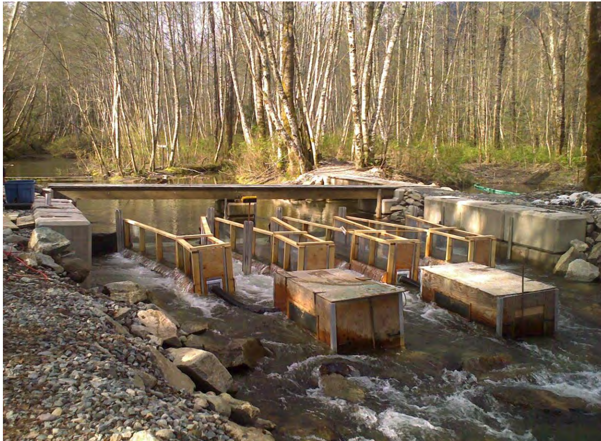
Figure 6. Upper Paradise Gorbushca (Site 1) Smolt Trap used to enumerate coho and steelhead smolts on the Cheakamus River side channel.
