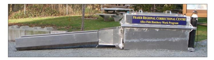
Figure 5 Sockeye transport tank with release slide connected, January 2010
