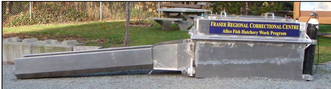
Figure 4. Sockeye transport tank with release slide connected, January 2010
