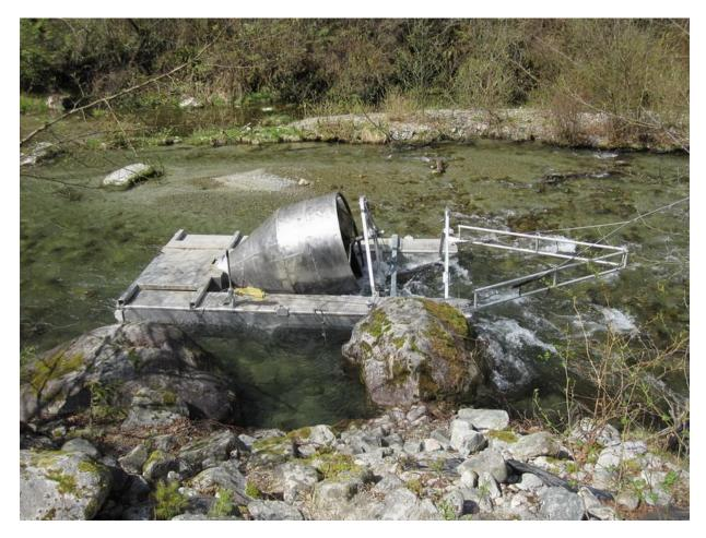
Photo 1. Mud Creek rotary screw trap, 14 April 2014.
