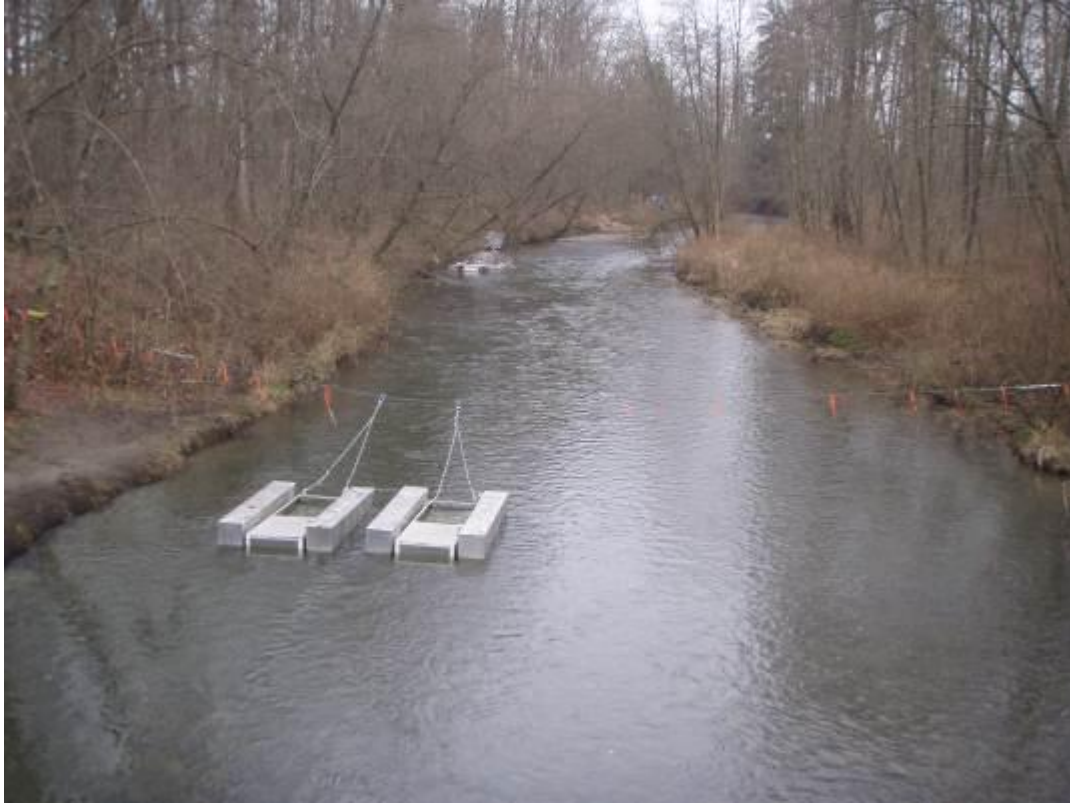
Figure 2.2. Photograph illustrating placement of the incline-plane traps. Note 1.8 m rotary screw trap in the foreground.
