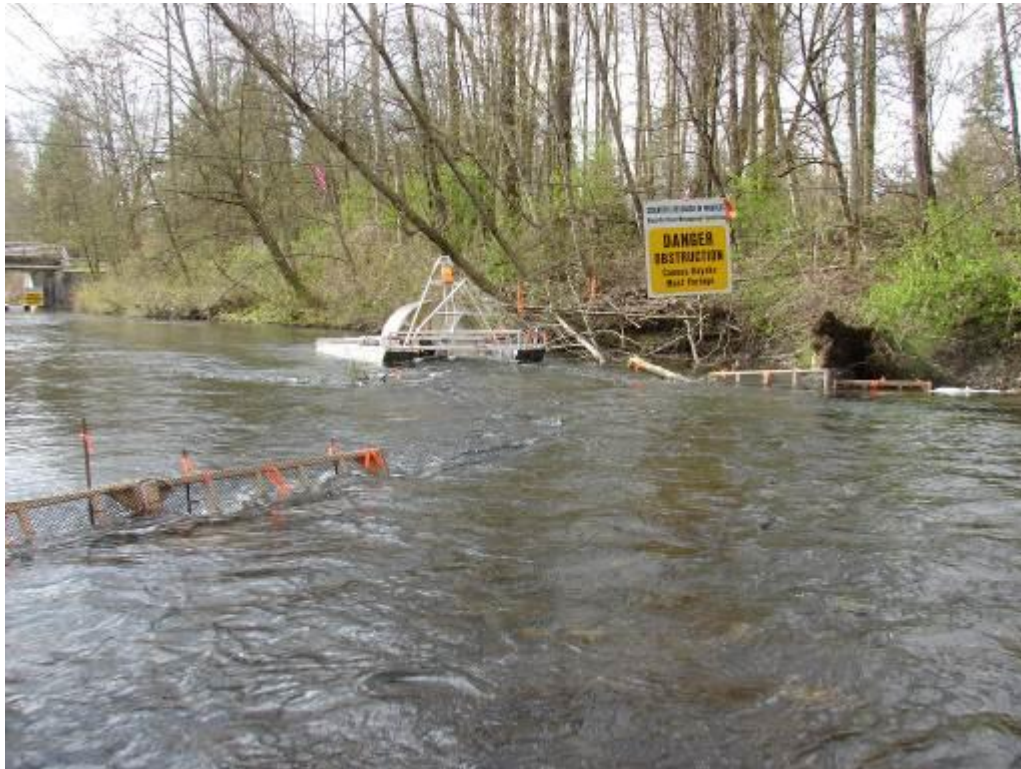
Figure 2.4. Typical 1.8 m rotary screw trap placement 14 April – 14 June. Note the use of screen panels and sandbags to concentrate flows and enhance trap efficiency.
