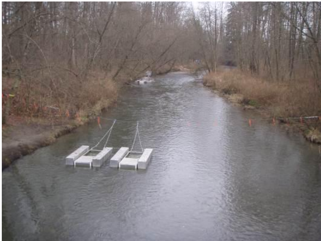
Figure 2.2. Photograph illustrating placement of the incline-plane traps. Note 1.8 m rotary screw trap in the background.
