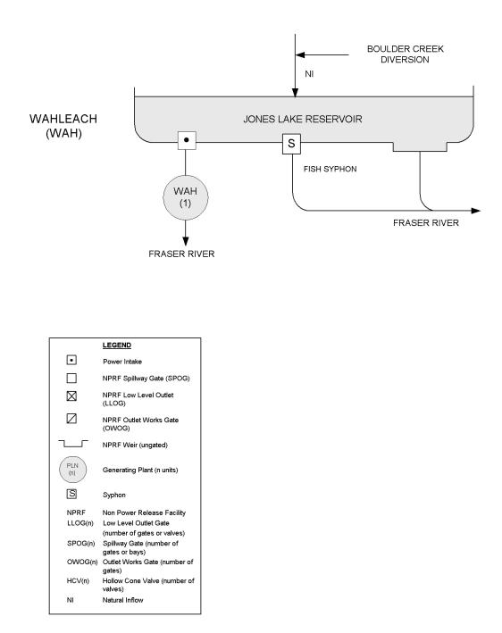
Figure 9: Schematic of the FLOCAL configuration for the Wahleach system
