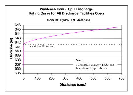
Figure 8: Rating curve for Wahleach Dam with all spill discharge facilities fully open
